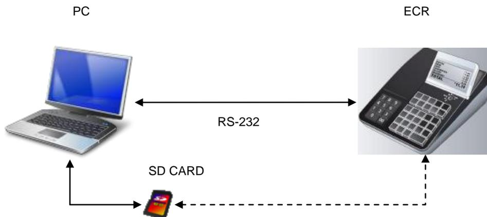
In case of RS-232, it can read and write ECR data directly by cable connection between ECR and PC
