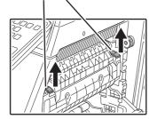
Lift the fusing unit pressure adjusting levers to allow easier removal.
