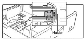
• When setting 8-1/2" x 11" size paper in tray 2, remove the 2 regulation plates with green colour on the front and back side of the tray before setting the paper. The plates are contained in the inside storage space of the back side of the tray.
