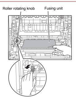
Carefully remove the misfed paper. Turn the roller rotating knob in the direction of the arrow to assist in removing it.
