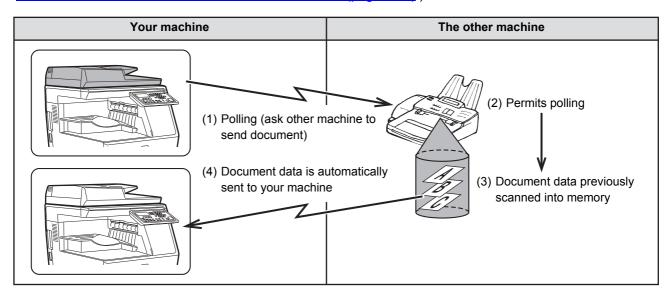
Group dials and the <u>SENDING THE SAME DOCUMENT TO MULTIPLE DESTINATIONS IN A SINGLE OPERATION</u> (page 4-30) can be used to successively poll multiple fax machines in a single operation (this is called "serial polling"). Up to 100 machines can be polled.
