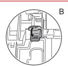
Return the lever to the normal position when finished feeding envelopes.
