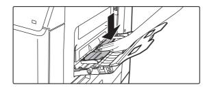
Push the centre of the pressure plate down until it locks into place.
