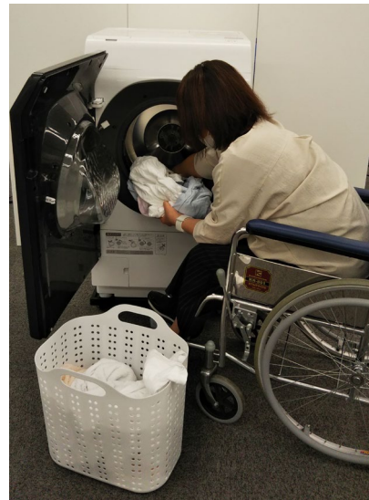
Evaluating the accessibility of a front-loading washer/dryer (for wheelchair users)
